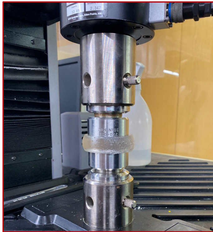
Figure 14. Compression of an Elastic50A sample cylinder on a MTS
