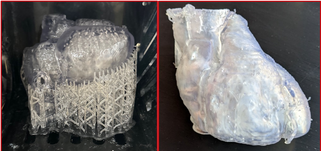
Figure 12. Whole heart 3D-print on the build plate (left) and after post-processing (right).
